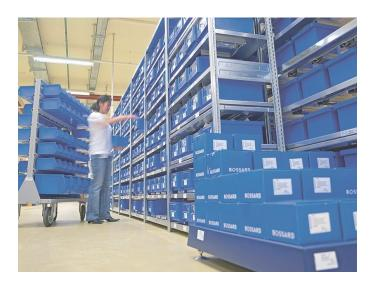
This unique, fully automated system with sensor monitoring is ideal for supermarket area and line assembly. SmartBin manages anything from small parts weighing just a few grams to large parts up to 2,000 pounds per pallet. Weight sensors ensure continuous inventory monitoring. Orders are triggered automatically and enable a seamless supply.
